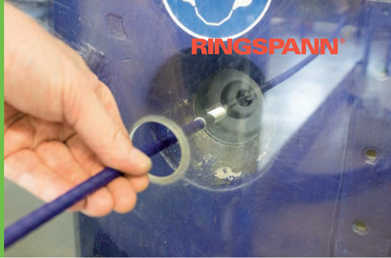
Rotary pressing of hose sleeves: RINGSPANN RCS also devotes great attention to pressing the end parts of its push-pull cables. An optimised press design is always used for each cable type.
