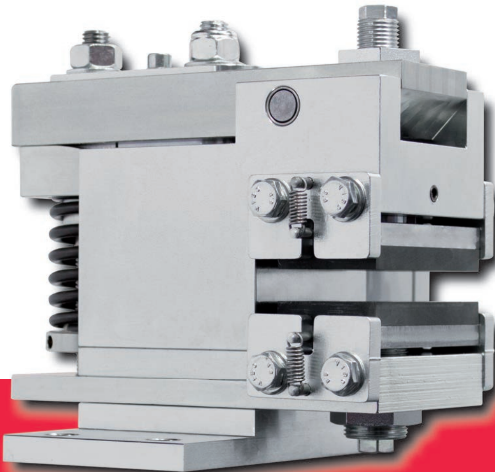
The electrical disc brakes of RINGSPANN. They achieve clamping forces of up to 24 kN and are suitable as holding or emergency stop systems for many industrial applications. The figure depicts a EV024FEM-type brake.
