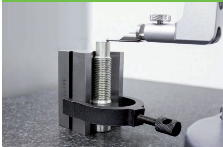
The quality assurance is a key factor in the mechanical cable production of RINGSPANN RCS. The illustration shows the measurement of a conduit cap.
