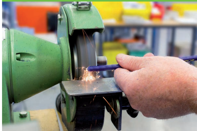
A look at production: The manual deburring ranks among the key quality factors in the push-pull production of RINGSPANN RCS. Many other manufacturers leave out this process step for cost reasons.
